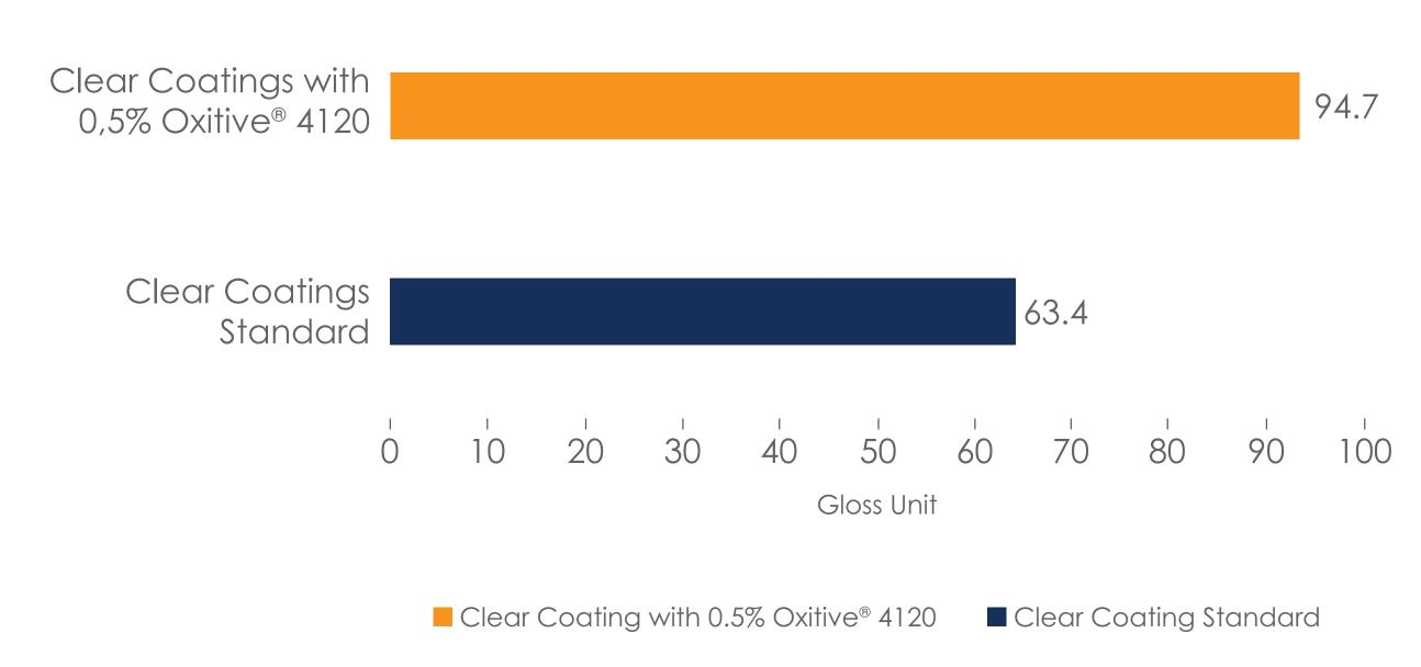
Method: Measurements determined with Gloss Meter according ASTM D 523-14 on Polyester Clear Coating applied to the steel sheet in a painting booth.
