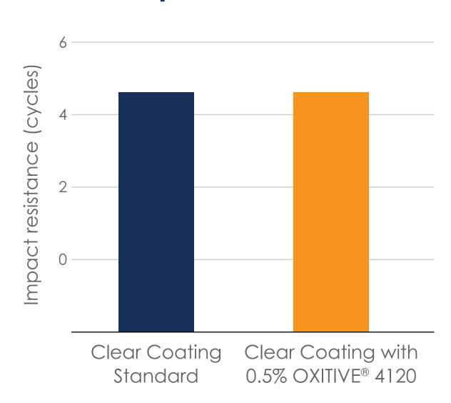
Method: Measurements determined according ASTM D6905-20 with Polyester Clear Coating / Basecoat / Primer applied to the steel sheet in a painting booth.
