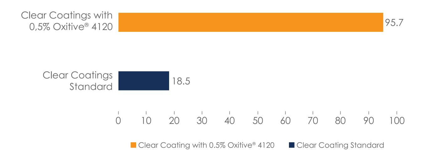
Method: Measurements determined according ASTM E 284 – 91 on Polyester Clear Coating applied to the steel sheet in a painting booth.
