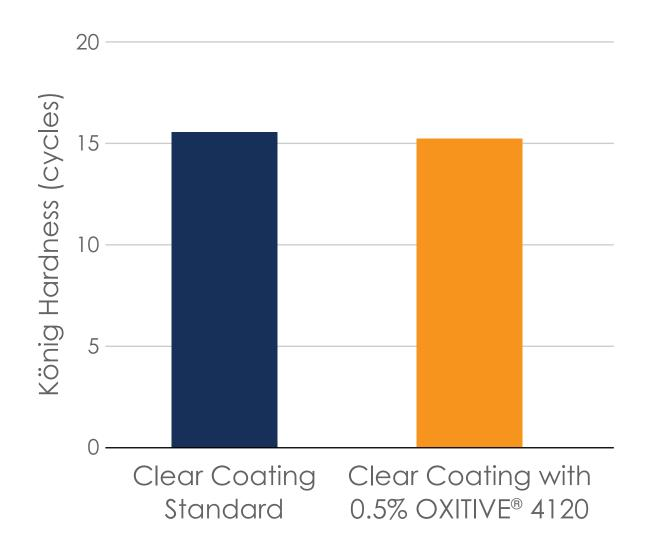
Method: Measurements determined according ASTM D4366 with Polyester Clear Coating / Basecoat / Primer applied to the steel sheet in a painting booth, after 10 days of cure in 25°.
