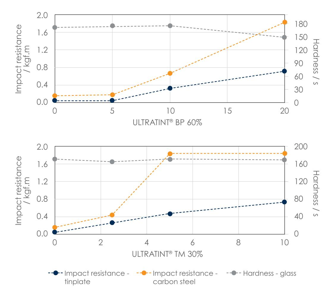
PU automotive top coating. ASTM D4366 and ASTM D6905.
