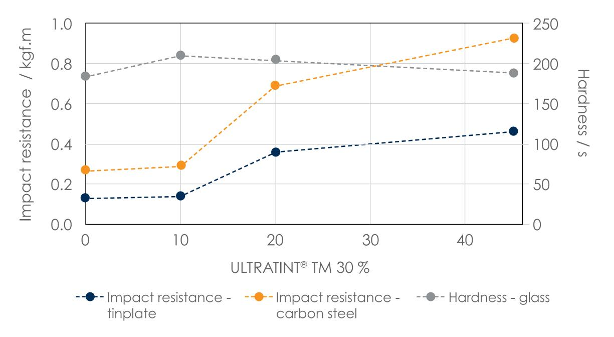
Polyester resine (%NV = 60.0 %, IOH = 5 %). Curing Agent: Aliphatic Polyisocyanate (NCO = 19.6%). R (NCO/OH) = 1.0. Methods: ASTM D4366 and ASTM D6905.
