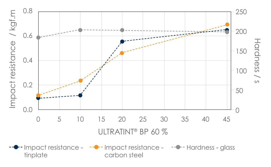
Polyester resine (%NV = 60.0 %, IOH = 5 %). Curing Agent: Aliphatic Polyisocyanate (NCO = 19.6%). R (NCO/OH) = 1.0. Methods: ASTM D4366 and ASTM D6905.
