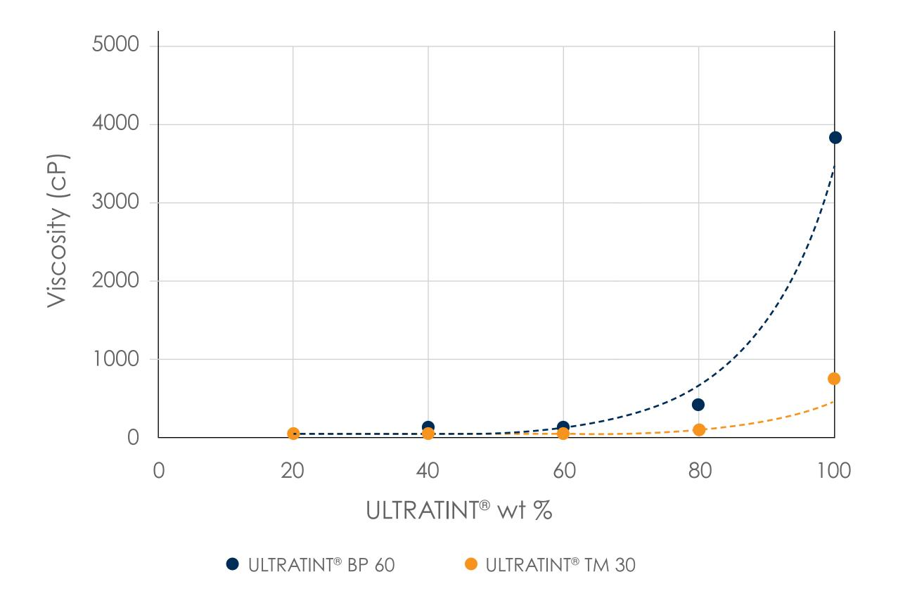
ULTRATINT® BP 60 or ULTRATINT® TM 30 can be added to aqueous medium up to 60 wt% with minimal increase in the viscosity of the system.
