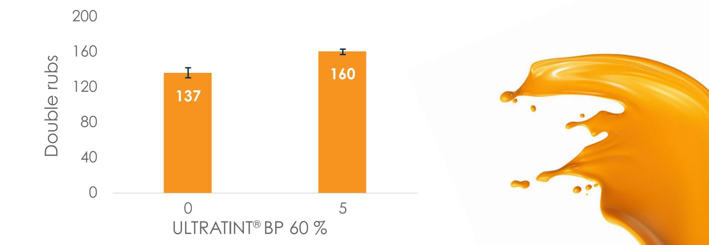
Acrylic resine (%NV = 50.0 %, IOH = 2.4 %). Curing Agent: Aliphatic Polyisocyanate (NCO = 19.6%). R = 1. Method: ASTM D5402.
