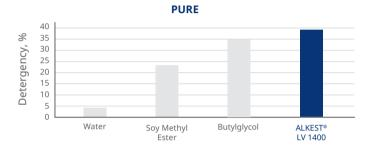
Soil: Stearic acid + Oleic acid + Carbon black | Surface: PVC tiles | Test method: Gardner Scrub | Formulation: 100% solvent
