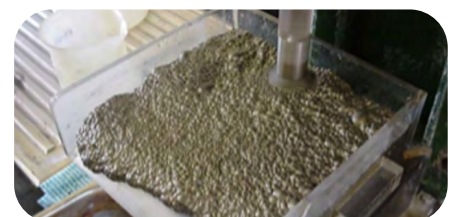
Nickel sulphide ore (high talc/MgO) with addition of 25 g/t of POLYMAX® T10
